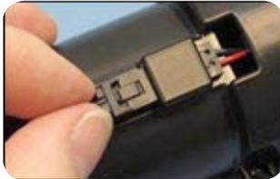
The battery is connected to VR2Tx on the side of the case. When installing the battery, listen for a "click" and watch that light flashes four times and then twice quickly every 5 seconds. When disconnecting battery, press the release tab on the battery connector and then pull connector halves apart.
