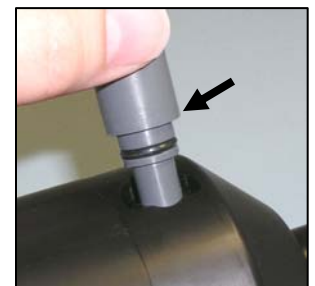
VRPC Interface probe being inserted into VR2.
