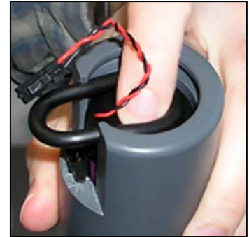
Inserting or removing the battery's O-ring
