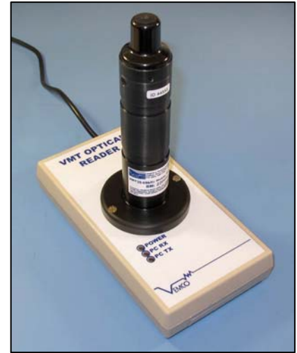
A VMT in the VMT Optical Reader
